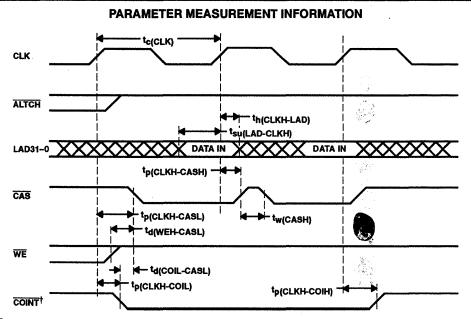
† COINT timing is for LADCFG high only. When the LADCFG bit is set high in the configuration register, COINT is controlled by bit 1 of the LAD move instruction instead of the set mask instruction.
