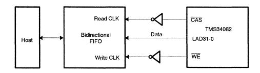
If LADCFG is set high in the configuration register, COINT defines bus cycle boundaries. If an indirect move to or from the LAD bus is coded with the C bit (bit 1) set high, COINT goes low at the beginning of the move and remains low until the move is complete. COINT can be used to select a device on the LAD bus, as shown in Figure 6–2. In this case, COINT is the output enable for a FIFO.
