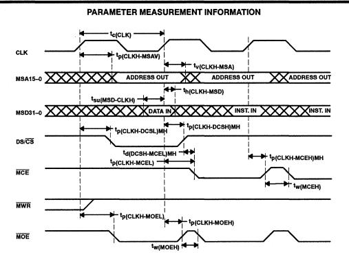
NOTE: This example shows a data read followed by an instruction read followed by an instruction read. This option for using DS/CS as data space chip enable and MCE as code space chip enable is invoked by setting the MEMCFG bit high in the configuration register. When MEMCFG is high, DS/CS and MCE rise after every rising clock edge. In this mode, DS/CS and MCE may not both be active (low) at the same time.
