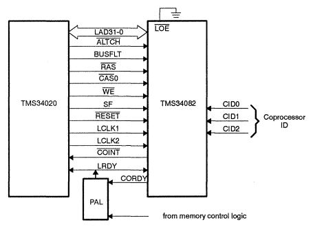
CORDY from the TMS34082 is logically ORed with other ready signals from the system to form the TMS34020 LRDY input ready signal. Note that LRDY connects to both the TMS34020 and the TMS34082 inputs.
