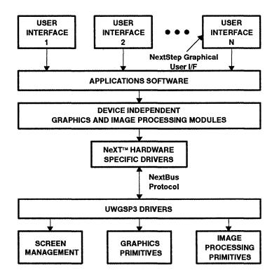
Figure 2. UWGSP3 Software Architecture
