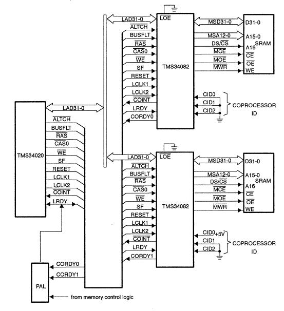
Figure 5–15. TMS34020 with Multiple TMS34082/SRAM Blocks (MEMCFG = L)
