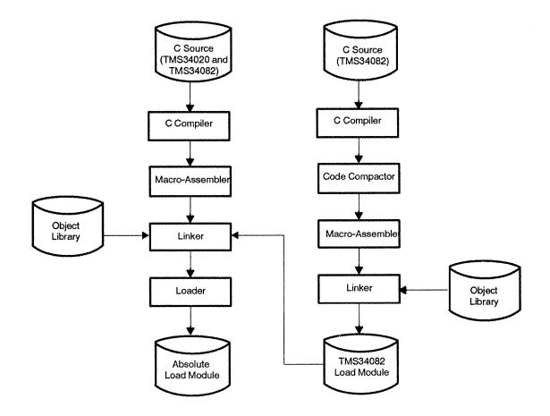
TMS340 Family Software Code Generation Tools (used for generating TMS34020 code and TMS34082 internal instructions)
