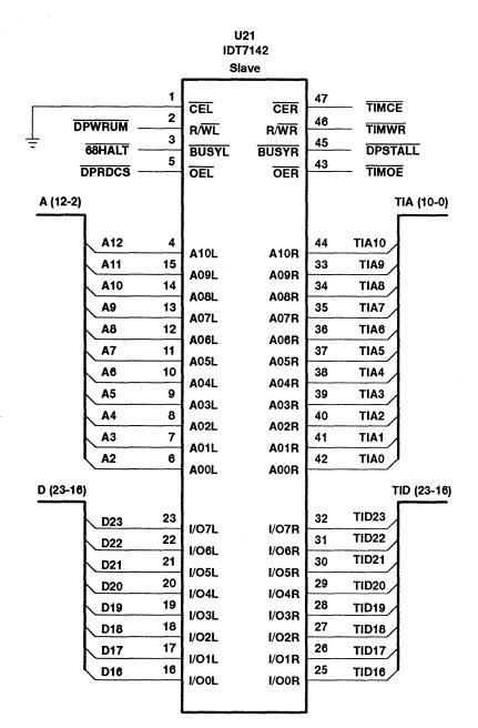
Figure 23. FIFO Logic, Details of U21
