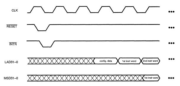
Loader operation begins on the second clock cycle after RESET and INTR return high. The first word is read into the configuration register on the rising edge of the third clock. Each successive rising edge loads an instruction word. The instruction word is output on the MSD bus one clock cycle after it is input on the LAD bus.
