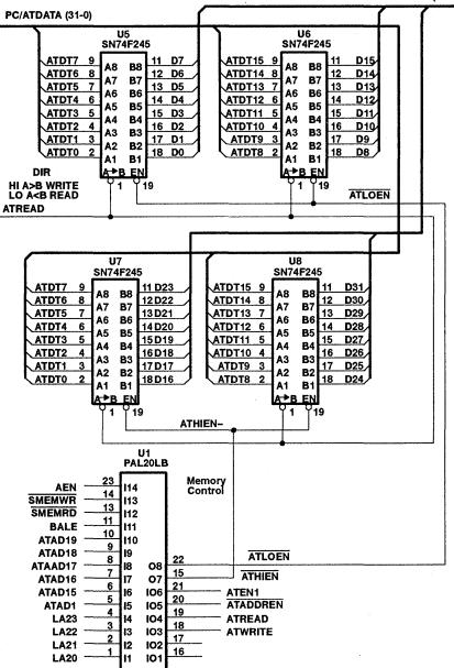
Figure 9. PC/AT I/F and Control, Details of U1, U5, U6, U7, and U8
