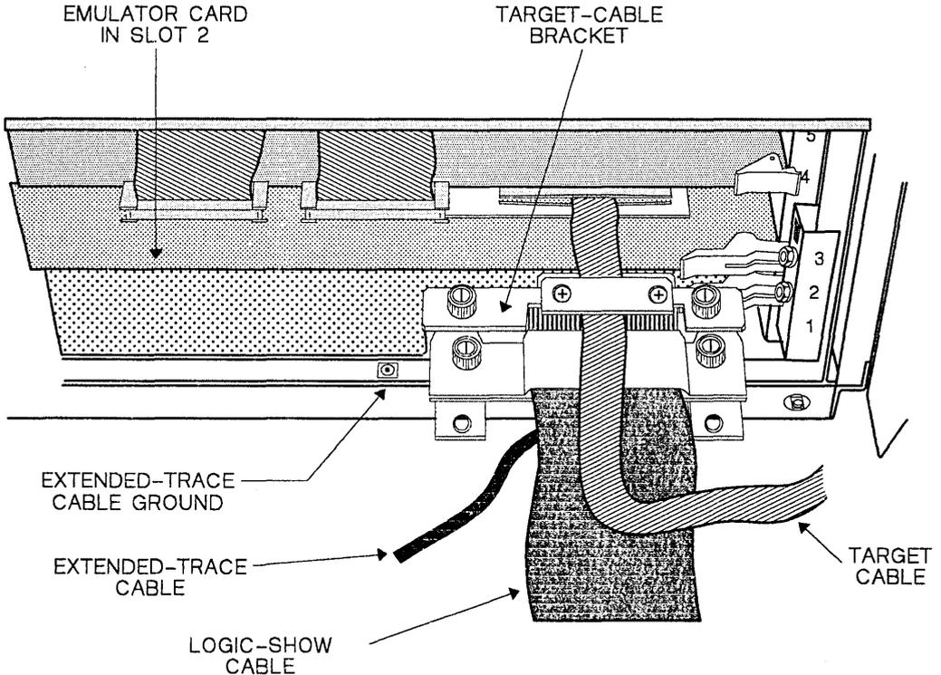
**Figure 11-3. TMS370 XDS/22 Complete Chassis Configuration**
