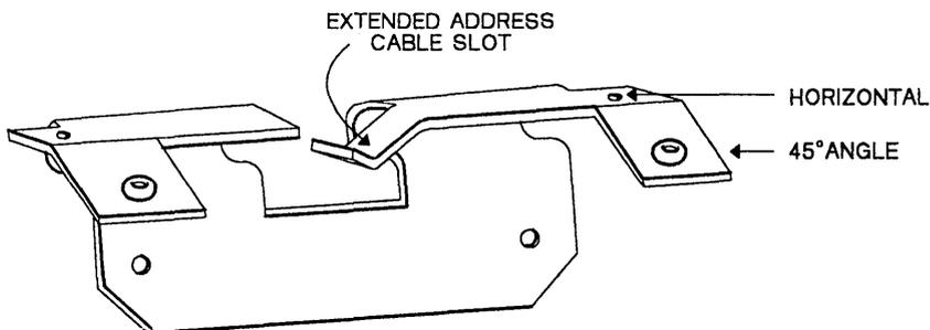
Figure 11-5. Chassis Cable Mounting
