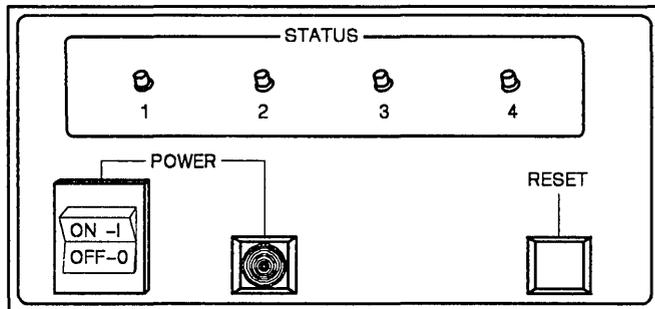
**Figure 11-1. XDS/22 Front Panel Controls and Indicators**
