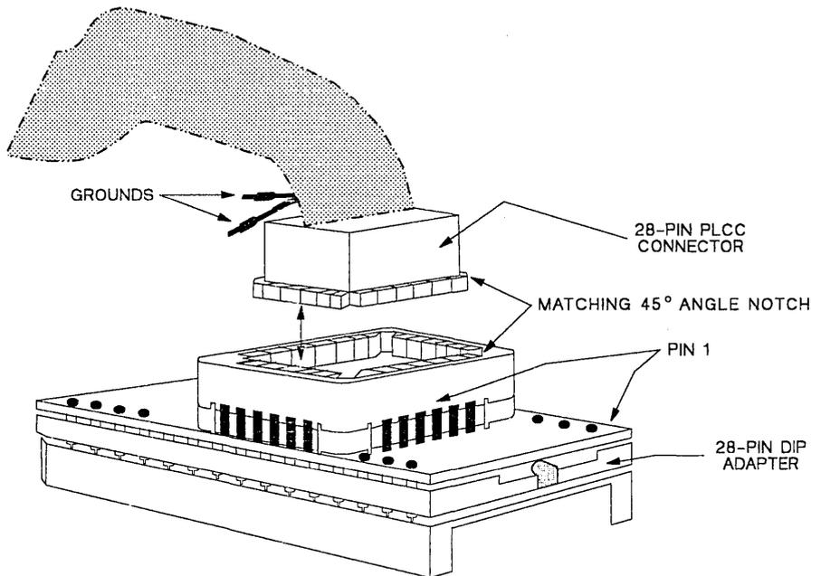
Figure 11-19. TMS370C010 Target Cable Assembly
