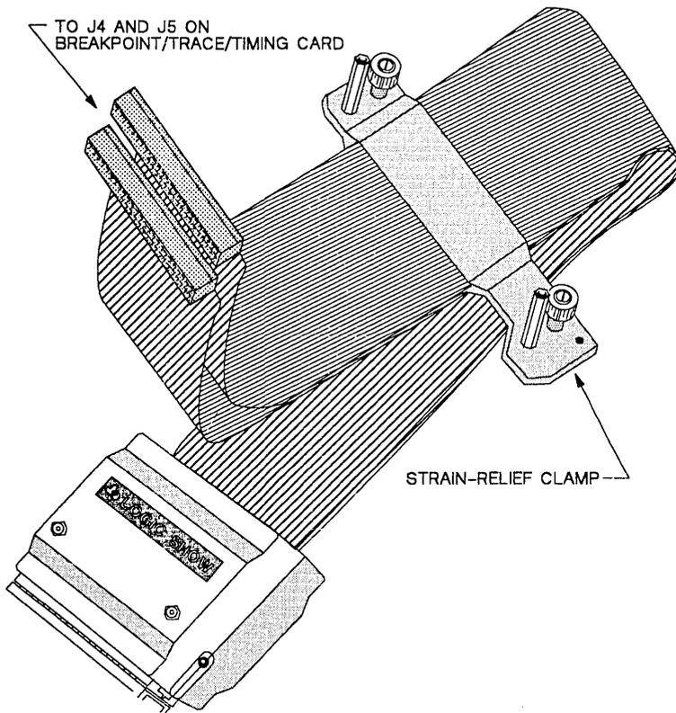
**Figure 11-13. Texas Instruments LOGIC-SHOW Cable**
