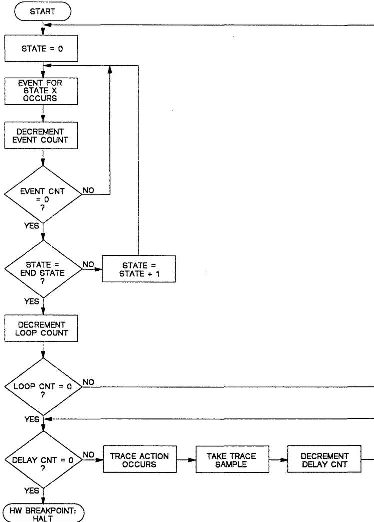
Figure 8-2. Flow of BTT Operation
