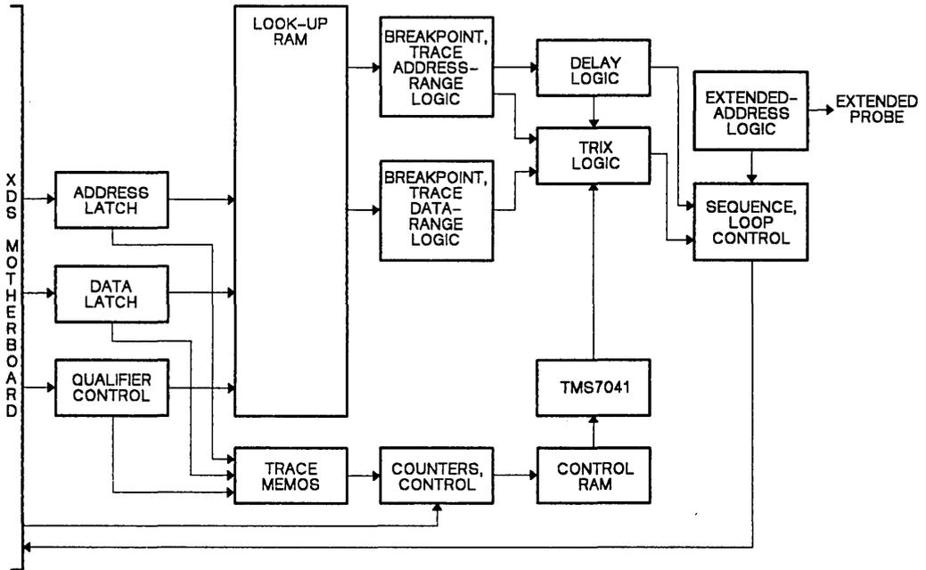
Figure 11-12. Breakpoint/Trace/Timing Card Block Diagram
