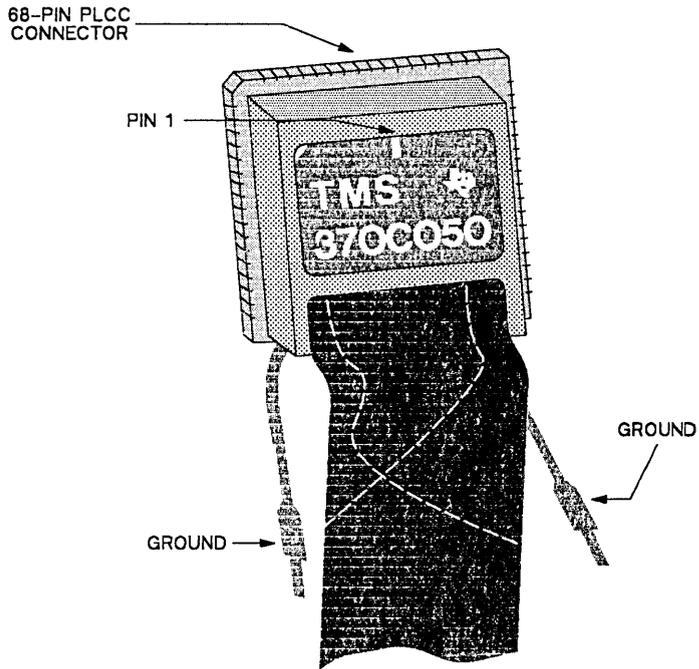
Figure 11-18. TMS370C050 Target Cable Assembly
