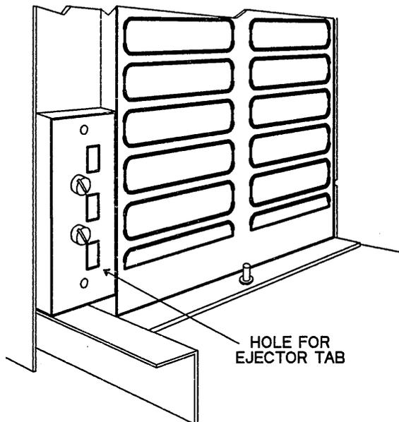
Figure 11-17. XDS/22 Card Cage Ejector Tab Holes
