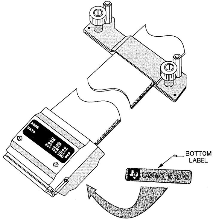
Figure 11-14. LOGIC-SHOW Cable Showing Pinout Label
