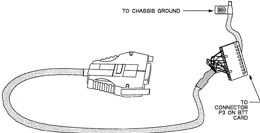
Figure 11-15. Extended-Address Cable
