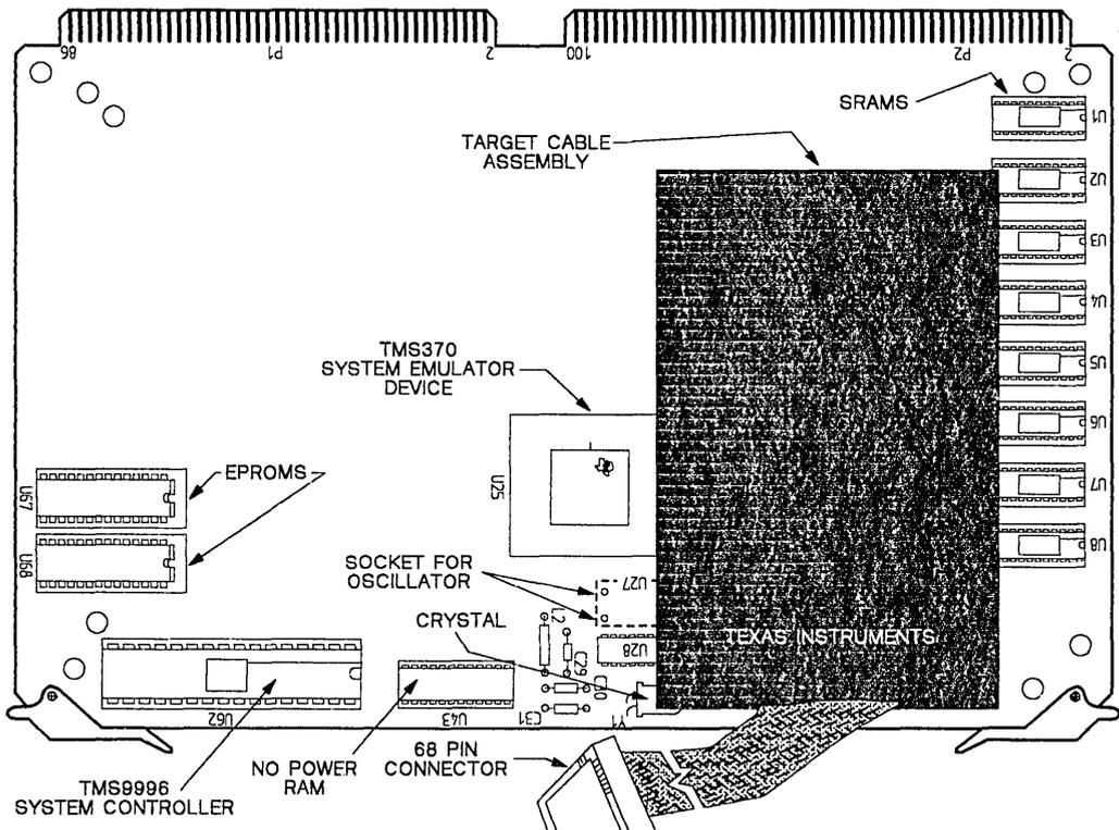
Figure 11-8. TMS370 Emulator Board with Target Cable Attached
