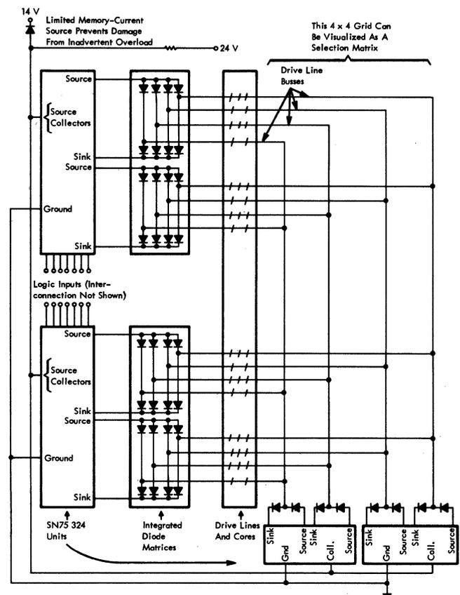
FIGURE 2. Typical Application of SN75 324 in Memory-Drive: A Selection Scheme for 16 Drive Lines
