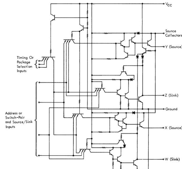
FIGURE 9. Schematic Circuit of SN75 324
