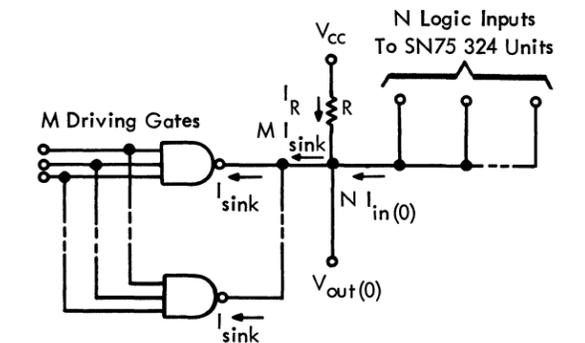
$$\text{Current in resistor} = I_R = M I_{\text{sink}} - N I_{in(0)}$$
