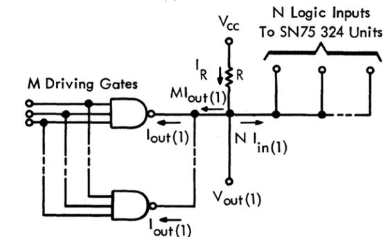
$$\text{Voltage across } R = V_R = V_{CC}(\text{min}) - V_{out(1)}$$
