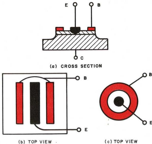
Fig. 3. Mesa-Type Diffused-Base or Double-Diffused Transistors
