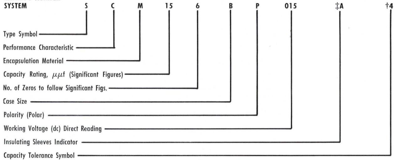
‡ The letter "A" in the second to last position of the Catalog number specifies no insulating sleeves. Change the letter "A" to the letter "B" for KEL-F insulating sleeves, or to the letter "D" for Mylar sleeves. Capacitors with flexible polyvinyl insulating sleeves available on request.
