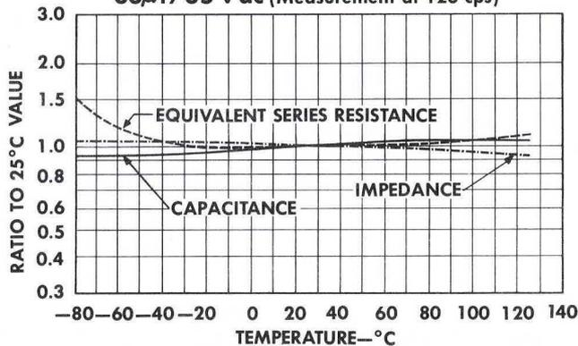
**IMPEDANCE, CAPACITANCE, EQUIVALENT SERIES RESISTANCE vs TEMPERATURE**
