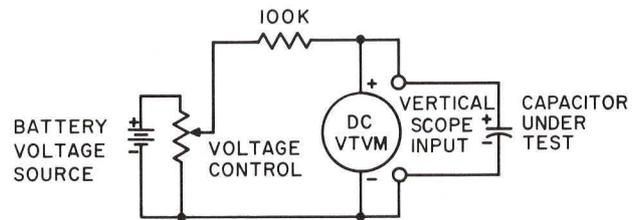
Oscilloscope has 1 megohm input impedance
