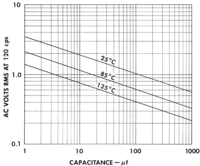
PERMISSIBLE RIPPLE VOLTS AC RMS vs
