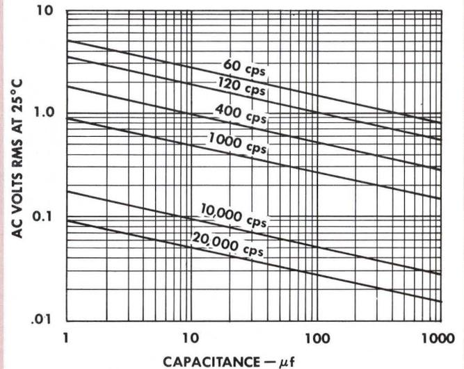
**a-c ripple voltage.** A capacitor type SCM may be operated with an impressed ac or ripple voltage provided the capacitor does not exceed its heat dissipation limits as established by the above charts. Total heat dissipation limits are affected by both the ambient operating temperature and the equivalent heating effect of the operating frequency as compared to the 120 cps test frequency.
