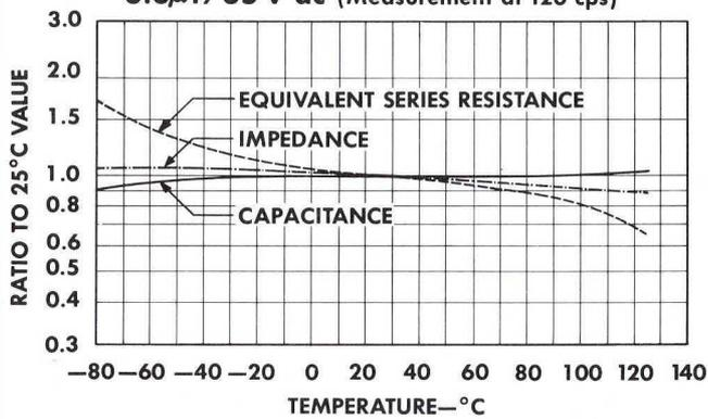
**IMPEDANCE, CAPACITANCE, EQUIVALENT SERIES RESISTANCE vs TEMPERATURE**
